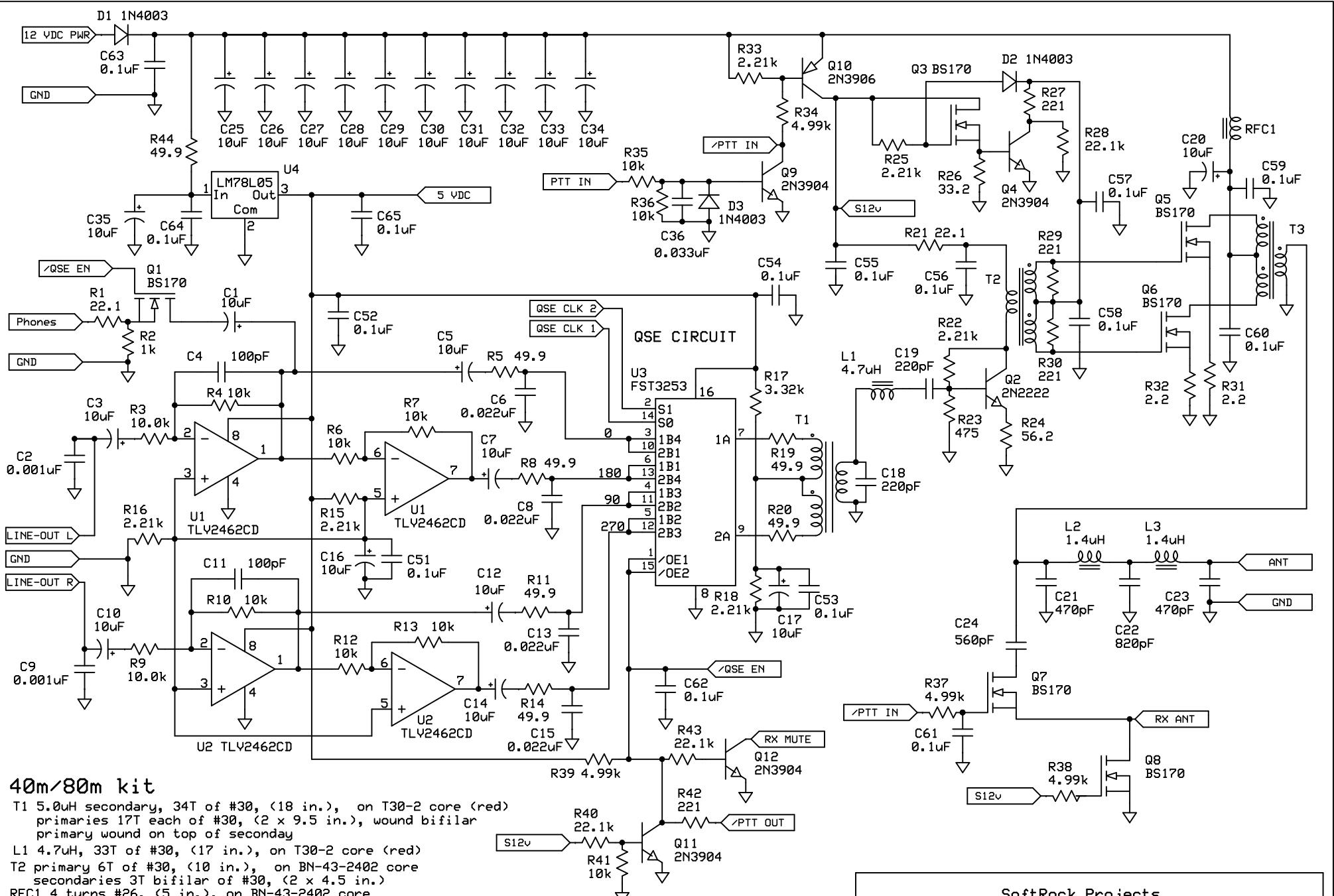
Note: Components mounted to the bottom of the board include size 1206 SMT capacitors C50 through C73 and SOICs U1, U2, U3, U5, U6, U7 and U8
